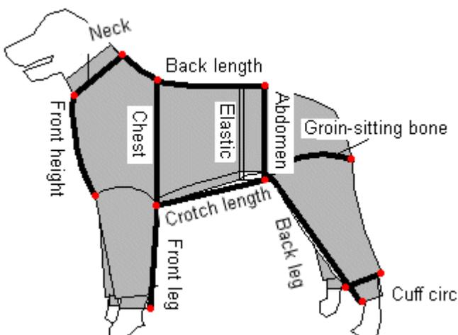
The front height and the leg measurements as well as the cuff circumference are garment measurements. Measure them as you want them to be in the ready garment. When measuring the leg lengths, **do not subtract** the height of the cuff ribbings, the macro does it for you.
